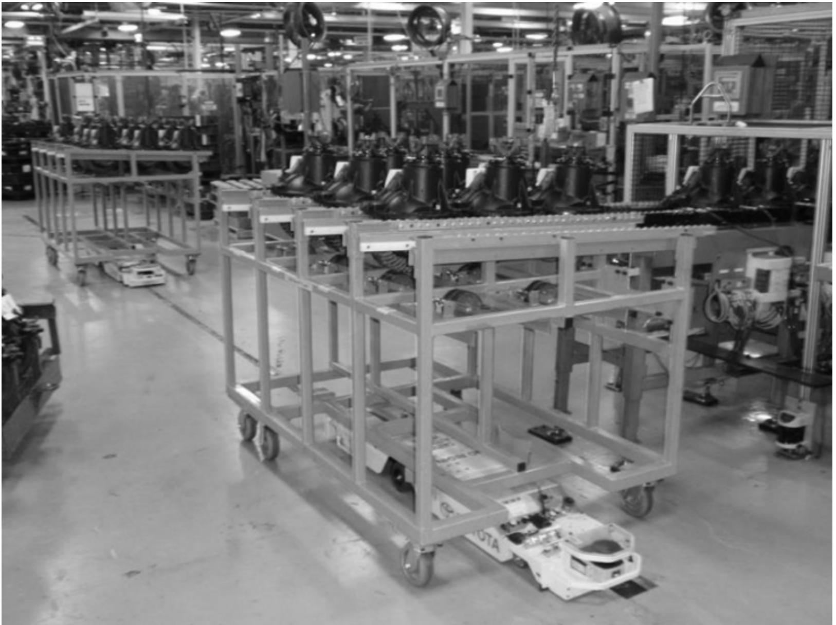
Figure 6-6. Automated Guided Vehicles bringing Axle Subassemblies with no Containers at Dana
